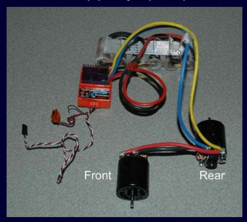
Notice how the wiring from the Electronic Speed Control is soldered to the rear motor. A common problem with this wiring setup is that the motor with the most amount of resistance stalls, typically the rear. By wiring up the rear motor first you are effectively provide power to that motor first thereby reducing the motor stall effect.
