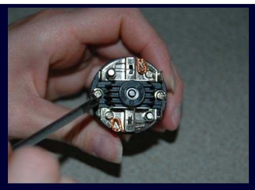
Once the can is marked you will then want to loosen the end bell screws.
