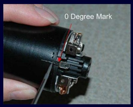
Once the can is marked you will then want to loosen the end bell screws.
