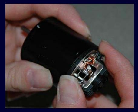
At this point you can then tighten the end bell screws to finish the process. Wiring...
