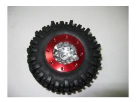
Install one screw at a time. Don't tighten the screw but a few turns. You can then install a screw directly across from the first. Once again, only a few turns. You will want to slowly install all the screws around the ring. Make sure the next screw is across from the previous screw. Just a few turns for each screw. (see the series of photos below)
