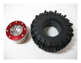
2. Remove the screws that hold the front and rear beadlock ring on the wheel. Keep track of all the screws you remove.
