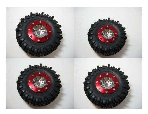
Now that all the screws are installed, you can begin to tighten them down. Following the same pattern that you used to install the screws, slowly tighten each one a few more turns. Then move onto the next screw. You need to do this until the screws are tight. Do not overtighten the screws, they can be stripped.
