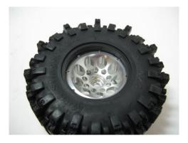
5. From one side of the wheel. Insert the tires bead into the groove of the beadlock wheel. (like in the photos below.)
