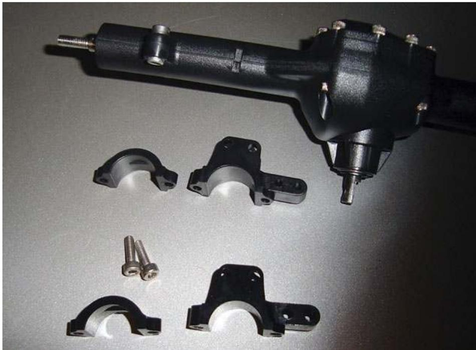
Here is the plastic mount fit onto the axle. These fit quite well, and seem to hold fairly strongly. I will note that the original pre-release plastic mounts were a bit weak and stripped easily, but RC4WD made the necessary changes to the plastic compound, and these final ones seem MUCH better! I should also mention that the **aluminum leaf spring mounts from RC4WD** will also fit these axles.
