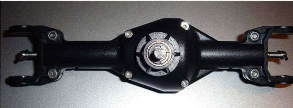
Note in the pictures above, that the axle is turned down at the ends far enough that the drive cups won't bind on the shafts. This will provide maximum steering possible! Below is about as much steering as you can get with no binding.
