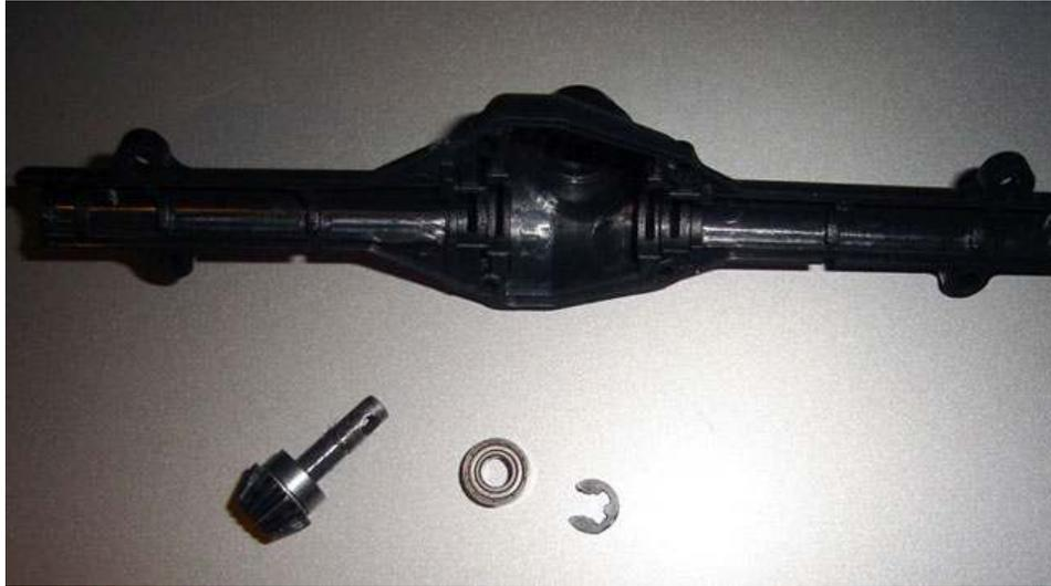
Here is the axle case with the bearings and pinion installed. It's worthy of noting that the shaft has a flat spot like most others, but is also pre-drilled for using the through-pins with Traxxas trype driveshafts. The 5mm shafts are perfectly sized for the smaller (Stampede, Rustler, etc.) Traxxas driveshafts. Anyone that's ever drilled a Tamiya pinion shaft will appreciate this little extra bit of work done for them. 😊
