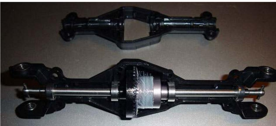
The front axle case is also held together by 4 M3 screws on the outer tabs, and 4 M2 screws at the center like the rear axle.
