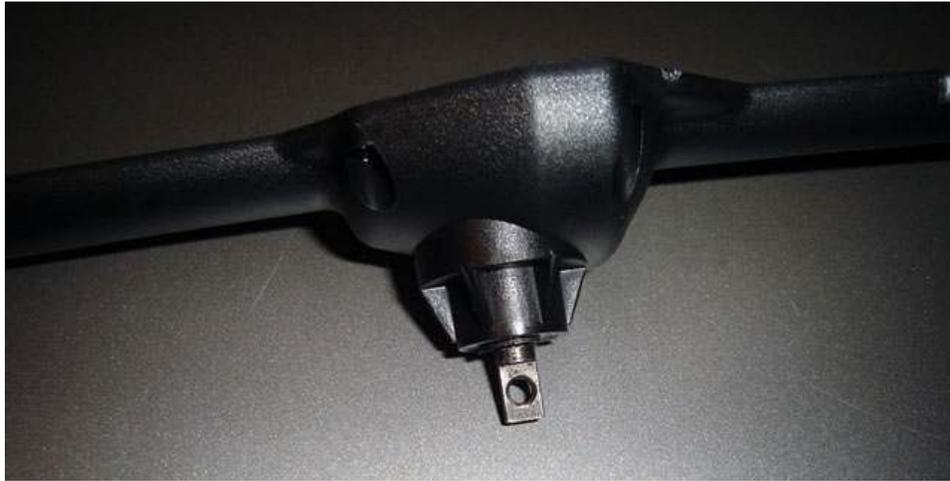
Here, is the same half of the case, with the spool and axle shafts in place. This is all designed like most other axles, with splines in the spool and on the end of the axle shafts, and E-Clips holding the shafts in place. There are two clips, one between the inner most bearing and spool on each side. Two 5x11mm bearings support each axle shaft. The spool is aluminum with a hardened steel ring gear. Seems to be pretty beefy! The gear ratio is 2.53:1 according to the specs on RC4WD.
