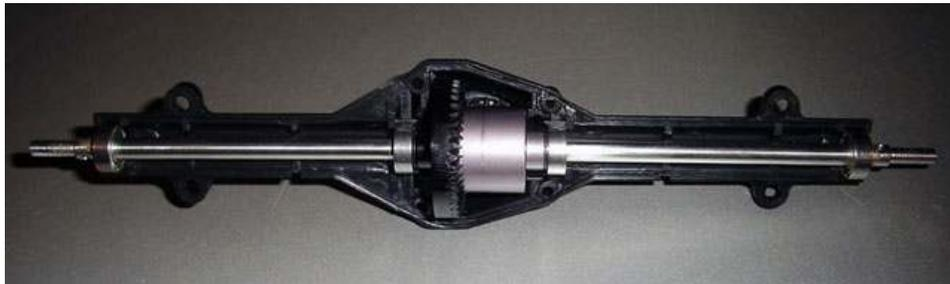
Now it's time to put the other half of the case on. The two halves are held together with 4 M3 screws and nuts on the tabs toward the ends of the axle, and 4 M2 screws that thread into the plastic at the center of the axle, as seen below.
