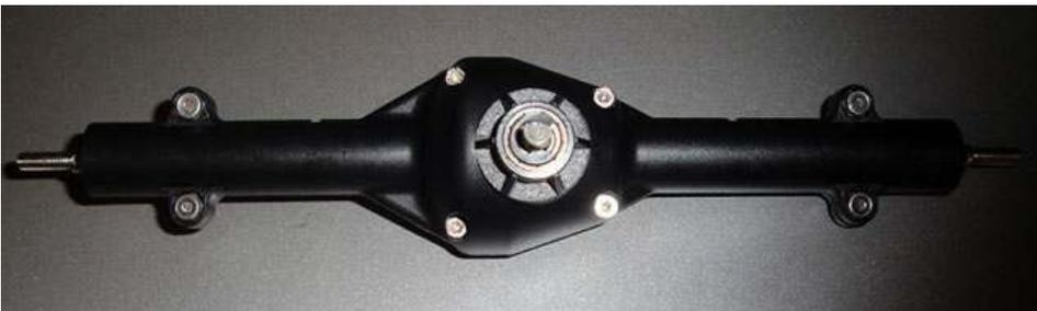
Now we can install the removable center diff cover. It is held on with 10 M2 screws for a nice scale touch. Nice!
